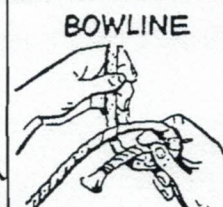
HOLDING ROPE WITH FINGERS ON TOP, PLACE END ON STANDING PART. TWIST YOUR HAND, CARRYING END AROUND TO FORM LOOP.
