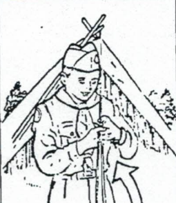
WHEN WHIPPING IS AS WIDE AS ROPE IS THICK, PULL OUT ENDS HARD. TRIM OFF TWINE CLOSE TO WHIPPING.
