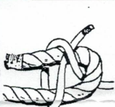
SHEET BEND FOR JOINING TWO ROPES TOGETHER OF DIFFERENT THICKNESS.
