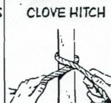
BRING ROPE END AROUND POLE, LAY IT OVER THE ROPE ITSELF.
