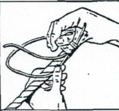
WRAP TWINE TIGHTLY AROUND ROPE STARTING 1/4 INCH FROM ROPE END.
